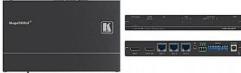
VM-3HDT is a high-quality, long-reach 1:3 HDBaseT extender distributor that takes one HDMI input, with IR and RS-232 control signals, converts it to an HDBaseT extension line signal and distributes it to 3 HDBaseT outputs that connect to compatible HDBaseT receivers. VM-3HDT includes an HDMI LOOP output for connecting to an additional unit in a daisy chain
